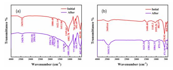
Fig. 6 FTIR of quartz (a) and magnetite(b) before and after adsorption with CTAC/lactic acid DES
