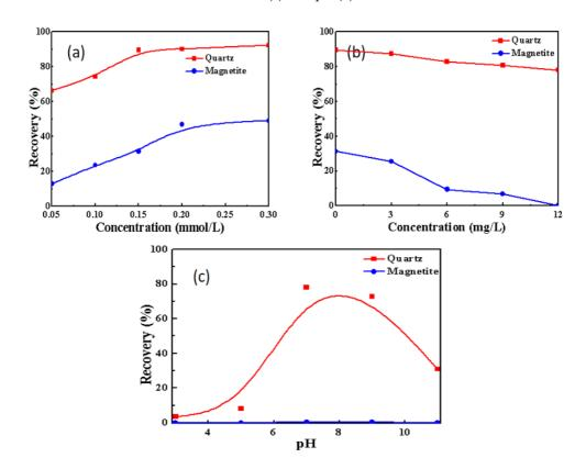
Fig. 5 The flotation recoveries of magenetite and quartz as a function of concentration of dodecylamine (a), concentration of starch (b) and pH (c).
