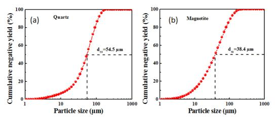
Fig. 1. Particle size distribution and cumulative distribution curve of quartz (a) and magnetite (b)
