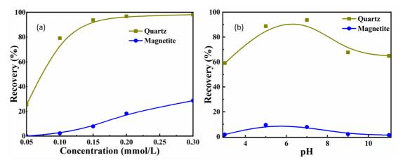
Fig. 4 The flotation recoveries of magenetite and quartz as a function of concentration of CTAC/lactic acid DES (a), and pH (b)
