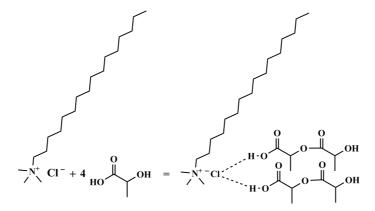
Fig. 2 The conceptual synthesis route of CTAC/lactic acid DES
